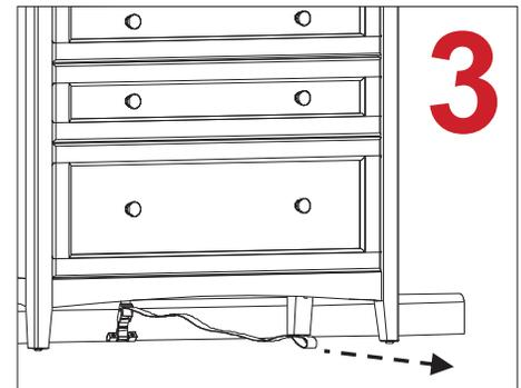
Push furniture against the wall and reach underneath to grasp the loop. Pull the loop end until tight.
