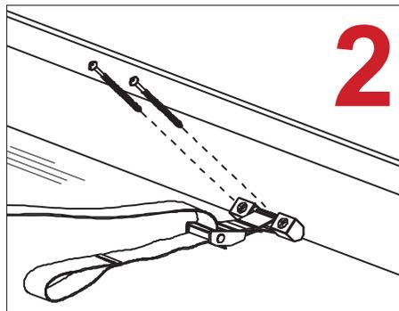
Loosen the strap and attach the bracket at a 45° angle under the baseboard in the desired location.
