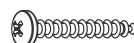
I — #8 x 20mm Pan Head Screw — Qty. 17 (inserted) (1356AFGAC; 1356AFCAF) — Qty. 22 (inserted) (1357AFGAC; 1357AFCAF) — Qty. 26 (inserted) (1358AFGAC; 1358AFCAF)
