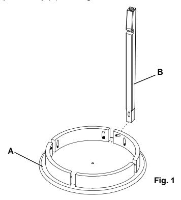
2. Using the pocket hole as a guide, secure the Leg (B) to the Top Assembly (A) with one #8 x 1-1/4" Pan Head Screw (E). See Figures 2 and 2a.
