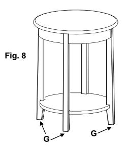
9. Place the table at its final destination. To level the table, rotate the Adjustable Glides (G) found on the bottoms of the legs. See Figure 8.
