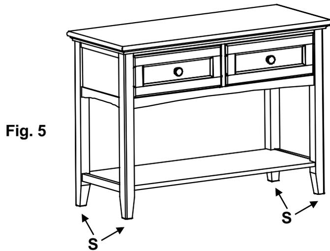
6. Place the table at its final destination. To level the table, rotate the Adjustable Glide (S) found at the bottom of each leg. See Figure 5.
