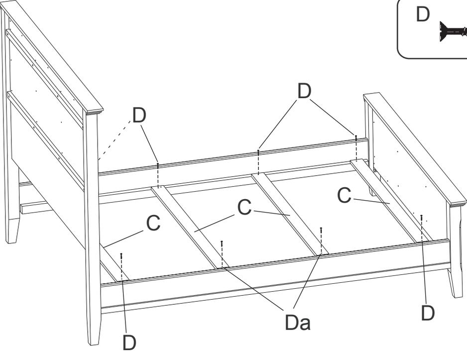
3. Position Slats (C) on bottom edges of rails as shown in Figure 3. Attach with 16 #8x1¼" Black Screws (D).
